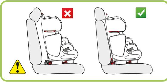
**Please note :** Position of adult seat belt head rest must not collide with car seat placed on the seat. It must be readjusted or removed if necessary.
