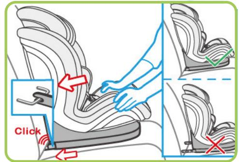
**Step 1.** Place the Child Car Seat on the car seat as forward-facing, adjust the backrest to the position higher than child's shoulder.
